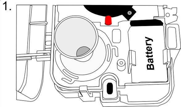
Install a 9V PP3 battery into the unit.
